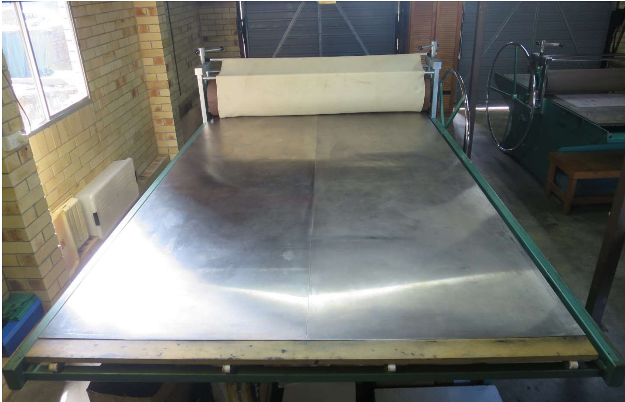
Figure 15 Large-format roller-style etching press, detail of 2m wide bed
