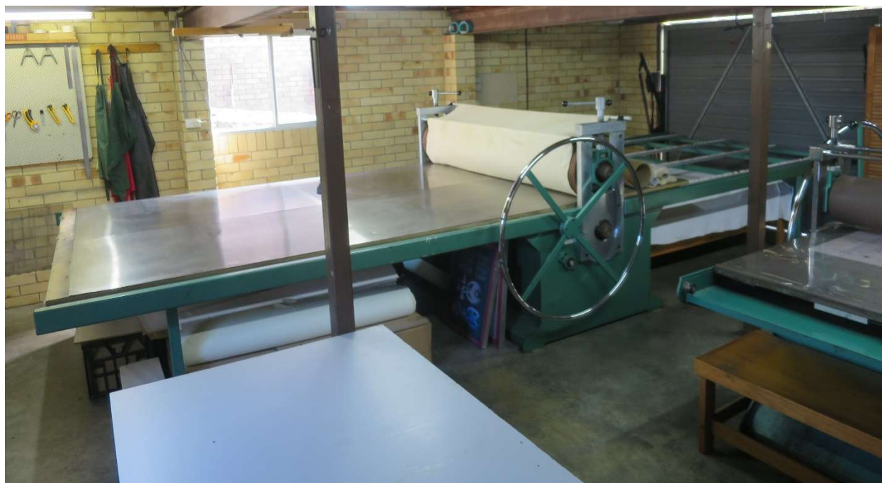
Figure 14 Large-format roller-style etching press
